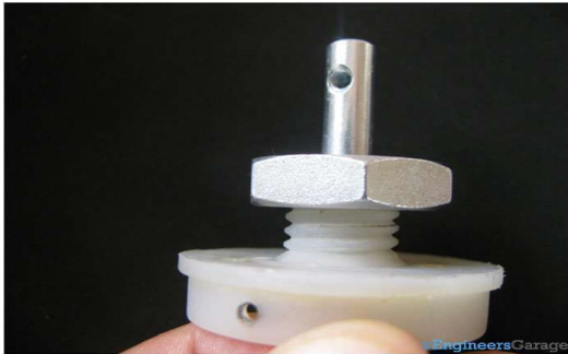
Fig. 3: Outer Structure of Gear Head DC Motor
