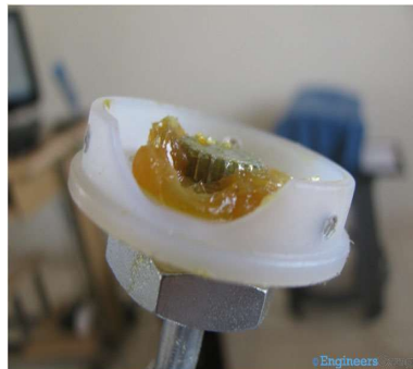
Fig. 7: Shape of Cap that Accommodates Gear
