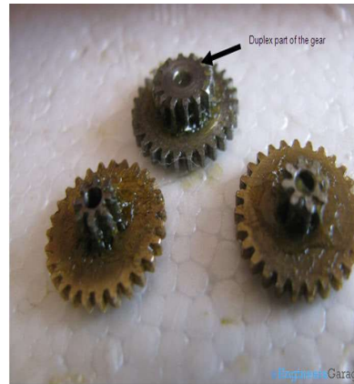
Fig. 12: Gears Shown Separately
