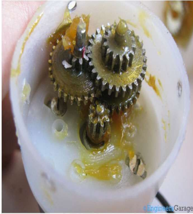
Fig. 8: Shape of Bottom Gear Assembly
