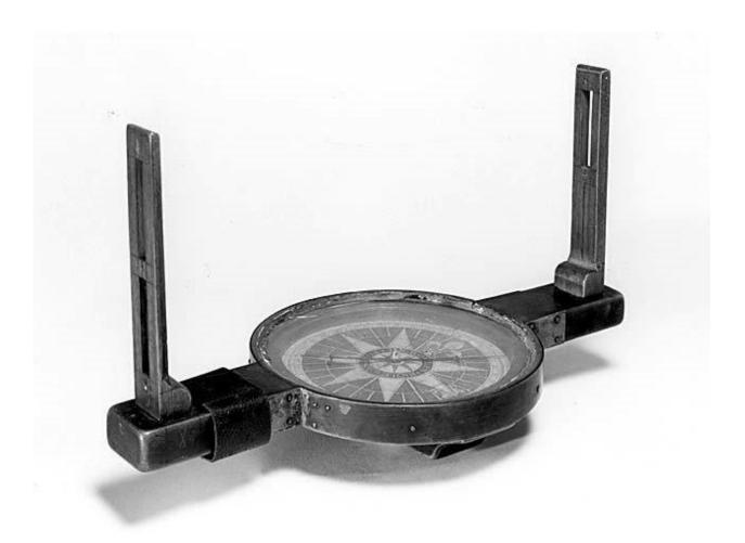
Like the prismatic compass for which Charles Schmalcalder obtained a British patent in 1812, this one lets the user read the card while sighting a distant object. It has a tall folding sight at north, and at south, a shorter sight with a prismatic eyepiece at its
