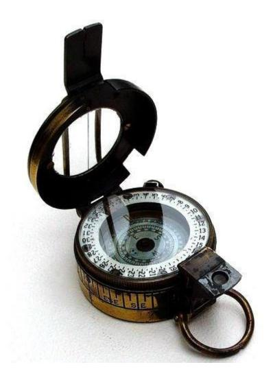
The survey which is based on the readings of learning takes with the help of a prismatic compass survey. In this survey the length of a line is measured with a chain or a tape. Thus the direction and length being known, the line can be easily plotted.
