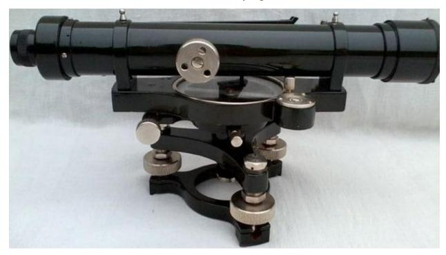
English civil engineer William Gravatt is considered as the inventor of the dumpy level. He invented dumpy level in 1832 while using the conventional Y level. A dumpy level is also called a builder's level, an automatic level.
