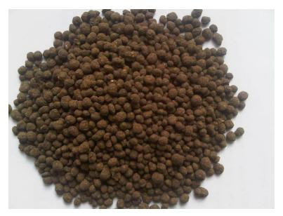
Press mud, the solid waste produced while processing sugar cane is rich in potassium, calcium, phosphorous and organic matters. Press mud is also a base material for producing bio-earth which is done by composting with spent wash, a liquid- waste generated out of distillery operation.
